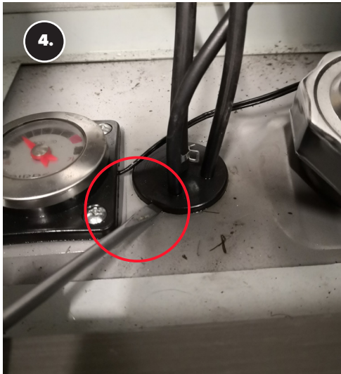
Remove the grommet with a screwdriver and lift it up.
